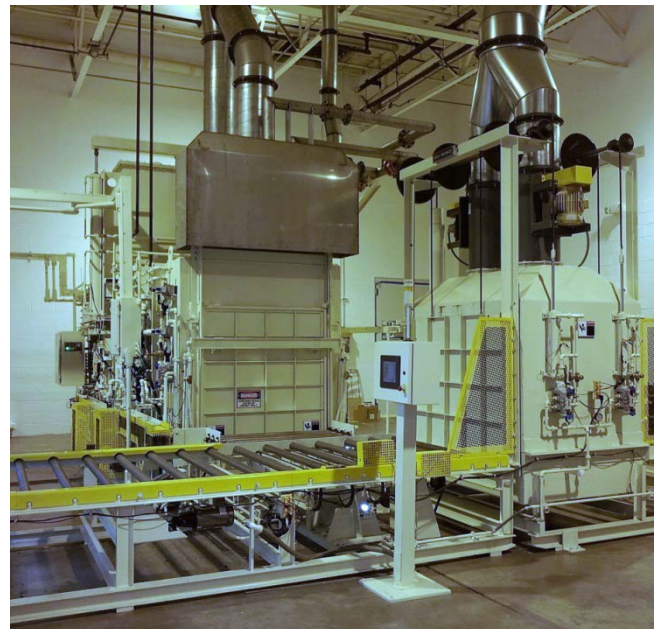
Fig. [9]. Universal Batch furnace. Load area size 1100 x 1100 x 1500 mm. Load mass 250 kg.
