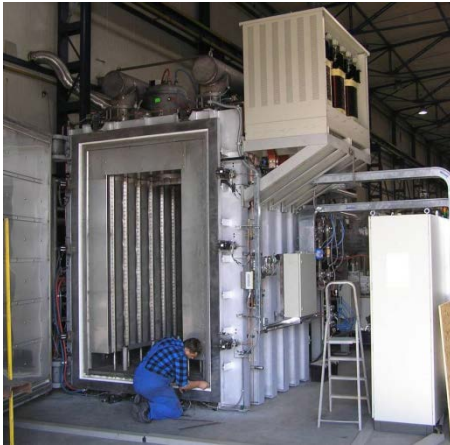
Fig. [10]. Single Chamber furnace with working area size 900 x 1900 x 2000 mm. Load mass 100 kg. Output - 1 cycle per hour. (SECO/WARWICK)
