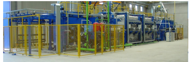
Fig. [8]. Semi Continuous High Volume furnace with vacuum purging at customer site. Load area size 250 x 2100 x 1350 mm. Load mass 400 kg. Output - 4 cycles per hour (SECO/WARWICK)
