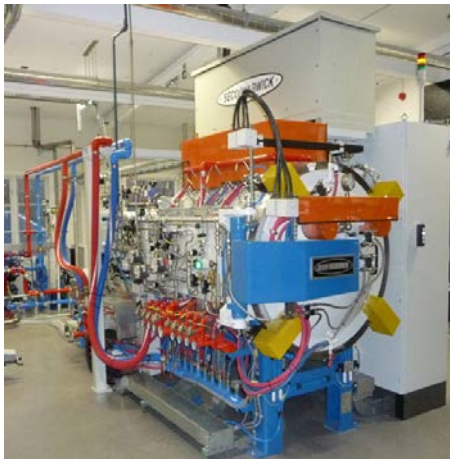
Fig. [11]. Single Chamber furnace with working area size 500 x 300 x 500 mm. Load mass 2 kg. Output 2 cycles per hour. (SECO/WARWICK)
