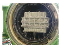
The load is supported on molybdenum rod inserts by graphite hearth rails running from front to back of the hot zone. Graphite piers from the cold wall chamber support the hearth rails.
