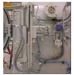
A hinged front door provides access for work loading, periodic cleanup and system maintenance. A lip seal located in a groove in the cover flange seals the flange-to-flange contact between the furnace chamber body and front cover, on closure of the vessel. Door clamp operated by linear motor allows positive pressure operations.
