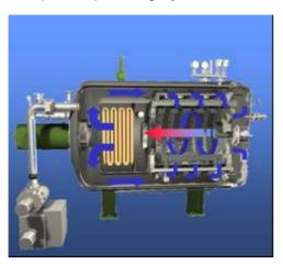
The cooling gas is injected uniformly onto the load through graphite nozzle arrays, which are deployed symmetrically in the hot zone cylinder and in the front insulation assembly. Special nozzle profile and high cooling gas velocity (up to 40 m/s) ensures excellent load space penetration and homogenous cooling. Hot gases escape the hot zone through a gas outlet bung in the rear wall.
