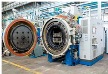
Figure 9: Pre-nitriding – single-chamber vacuum furnace system
