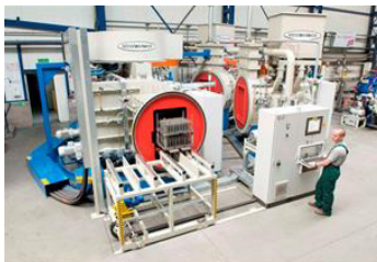
Figure 10: Pre-nitriding – multi-chamber vacuum furnace system
