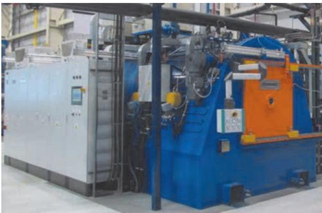
Fig. 1. Triple-chamber vacuum furnace for case hardening, type CaseMaster Evolution CMe T12
