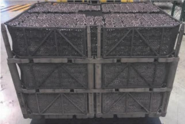
Fig. 4. Full batch for case hardening, 1200 kg, 35 m<sup>2</sup>
