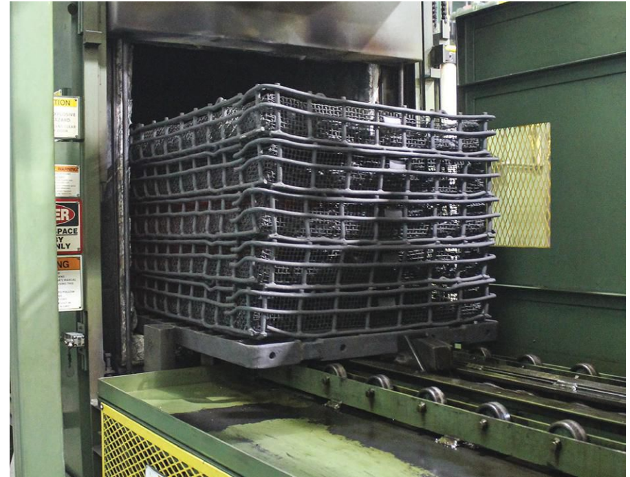
Fig. 1. Typical load exiting a tempering furnace (courtesy of MacLean-Fogg) tempered – subjected to a subcritical heat treatment that alters their microstructure and properties (Fig. 2). In general, tempering lowers strength and hardness while improving ductility and toughness of the as-quenched martensite. [3]
