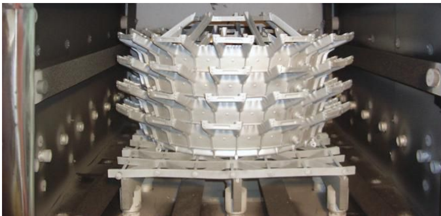
Fig. 1. Annealing of nickel-based alloy jet-fighter afterburner assemblies
