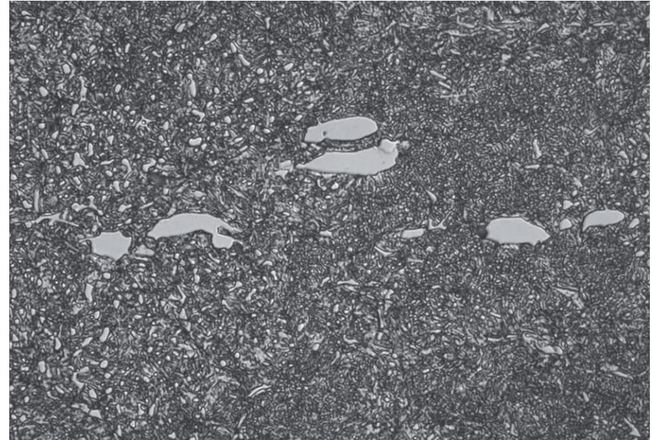
Fig. 2. A2 tool-steel microstructure – 1250X, 2% Nital (Courtesy of Aston Metallurgical Services Company, Inc.)
