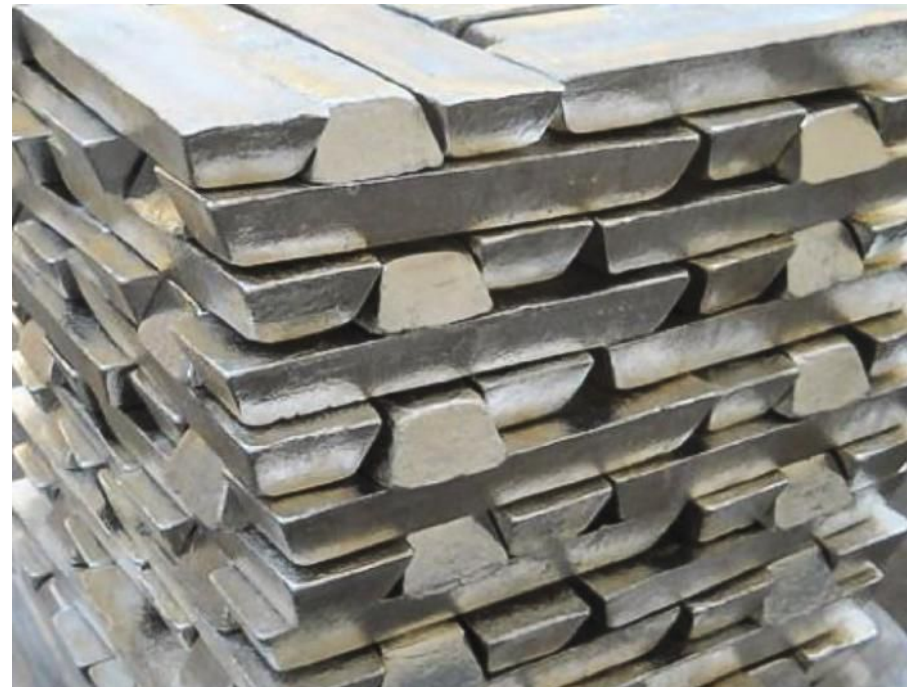
Fig. 1. Typical load of magnesium ingots [2]
