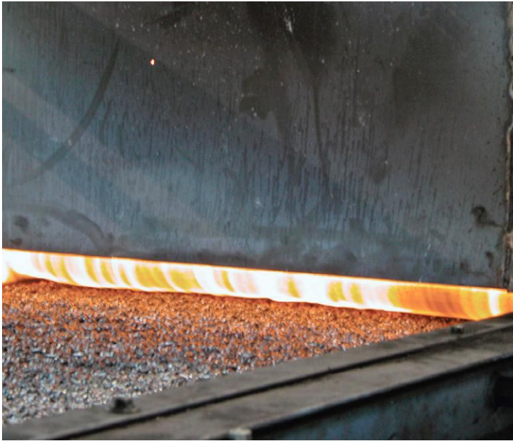
Fig. 3. Typical load of fasteners entering a mesh-belt furnace
