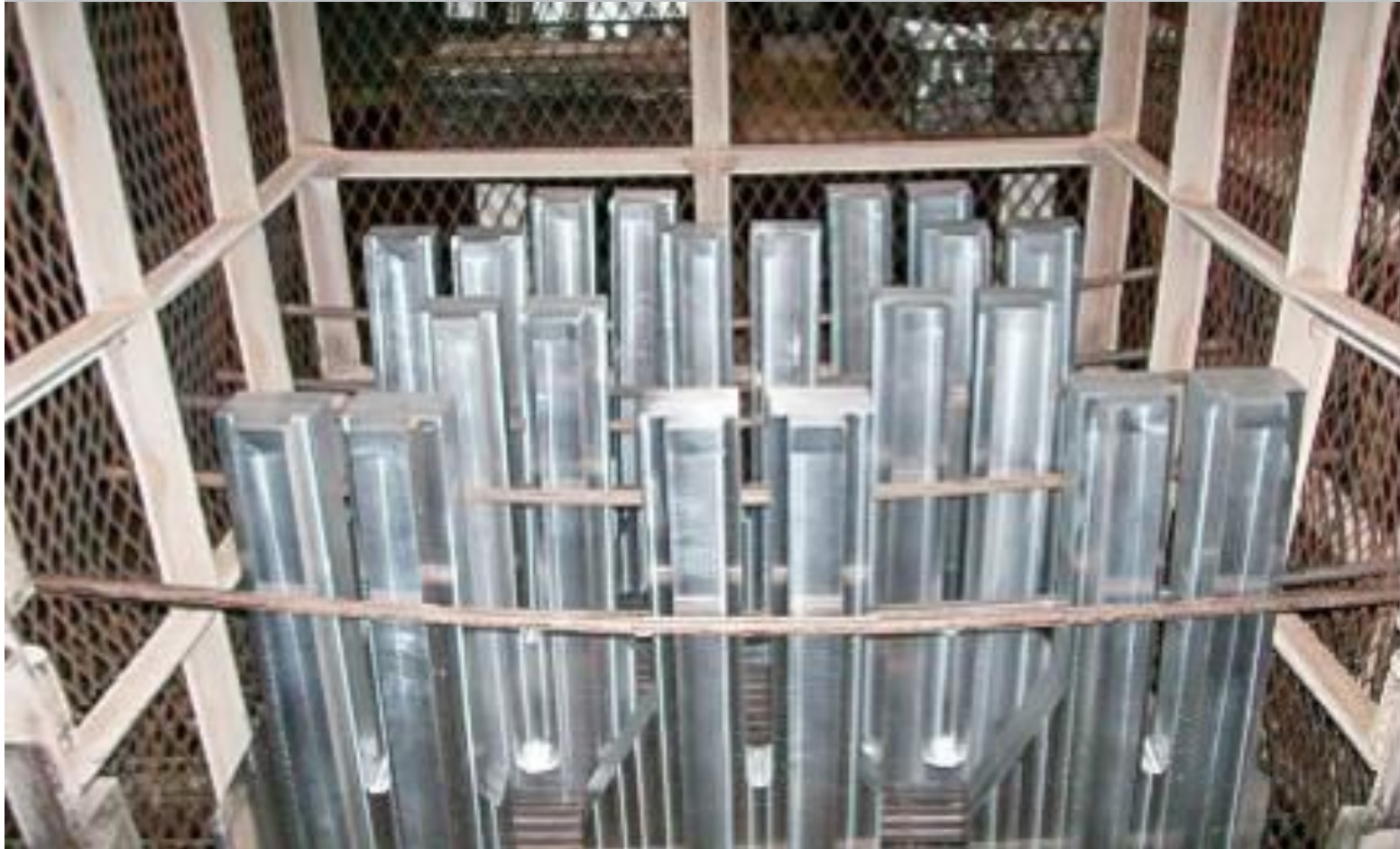
Fig. 1. Proper part racking
