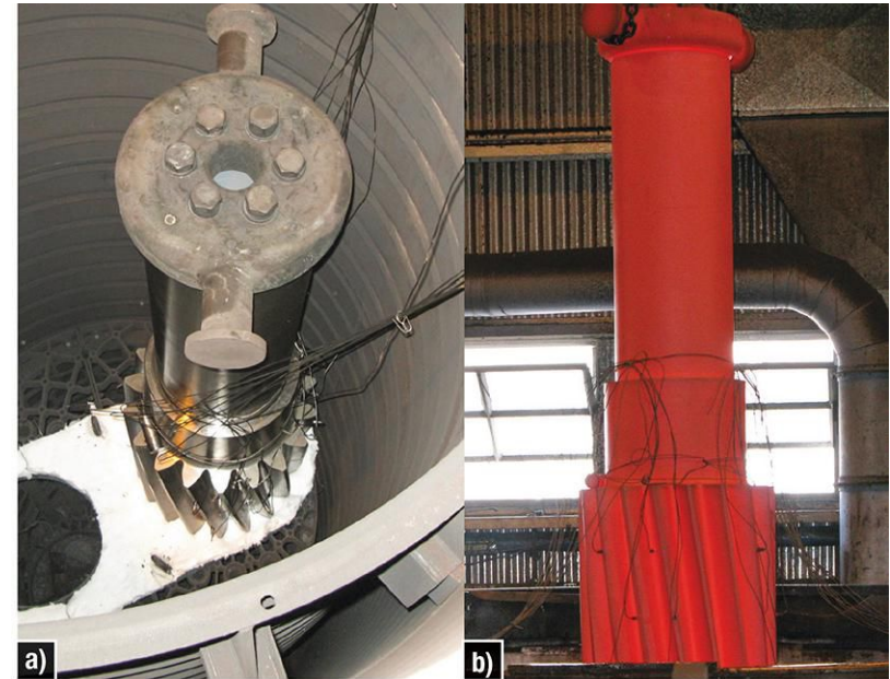
Fig. 3. Test part: (a) in position in furnace for heating test; (b) during transfer to the quench
