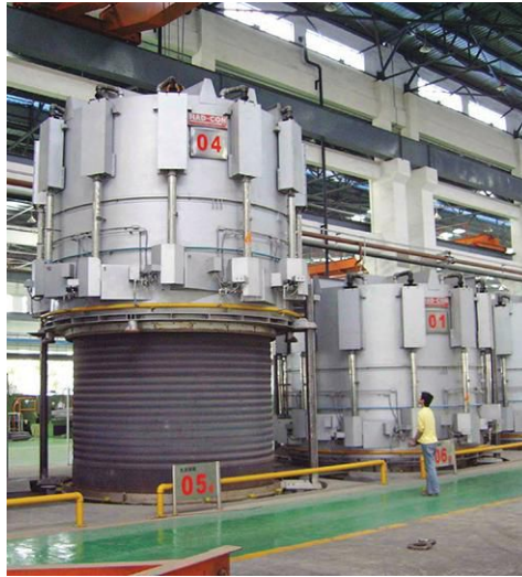
Fig. 3. Heating bell being lowered in place [6]
