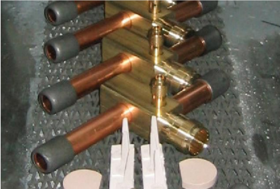
Fig. 8. Various ceramic temperature devices running with production parts
