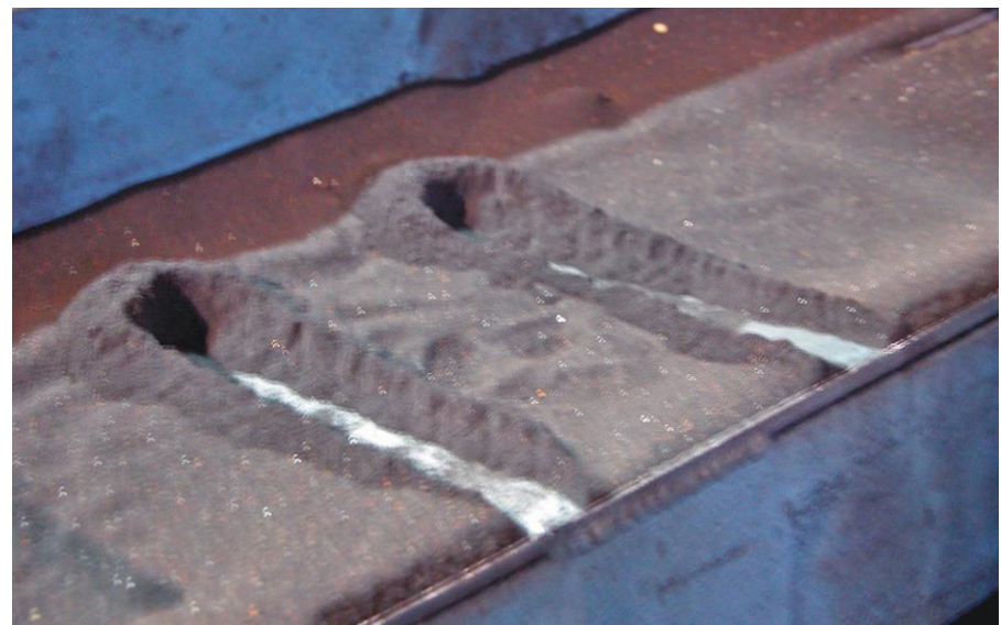
Fig. 4. Soot depositing on the front load table of a mesh-belt furnace after one hour with the furnace atmosphere out of control
