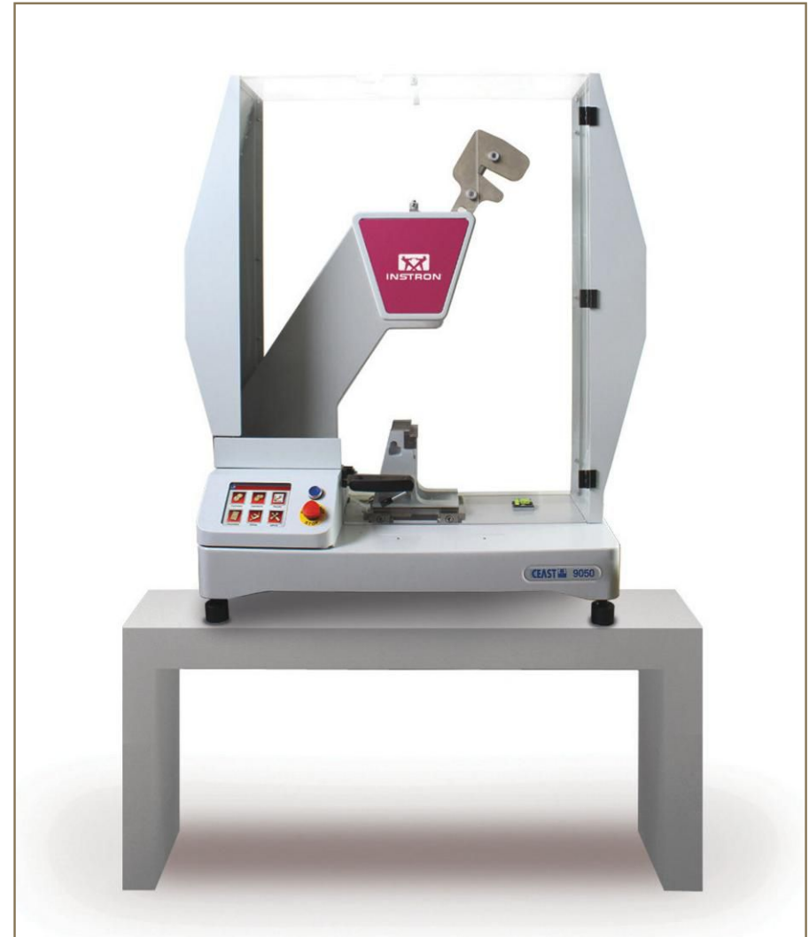
Instrumented impact tester (courtesy of Instron)
