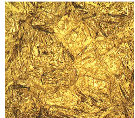
Fig. 5. Coarse martensite (carburized SAE 9310)
