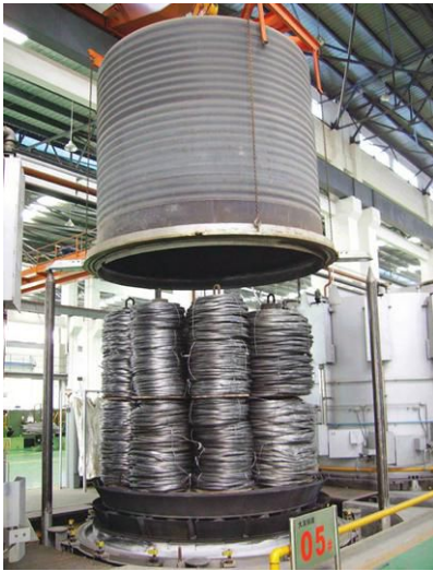
Fig. 2. Retort being lowered into position [6]
