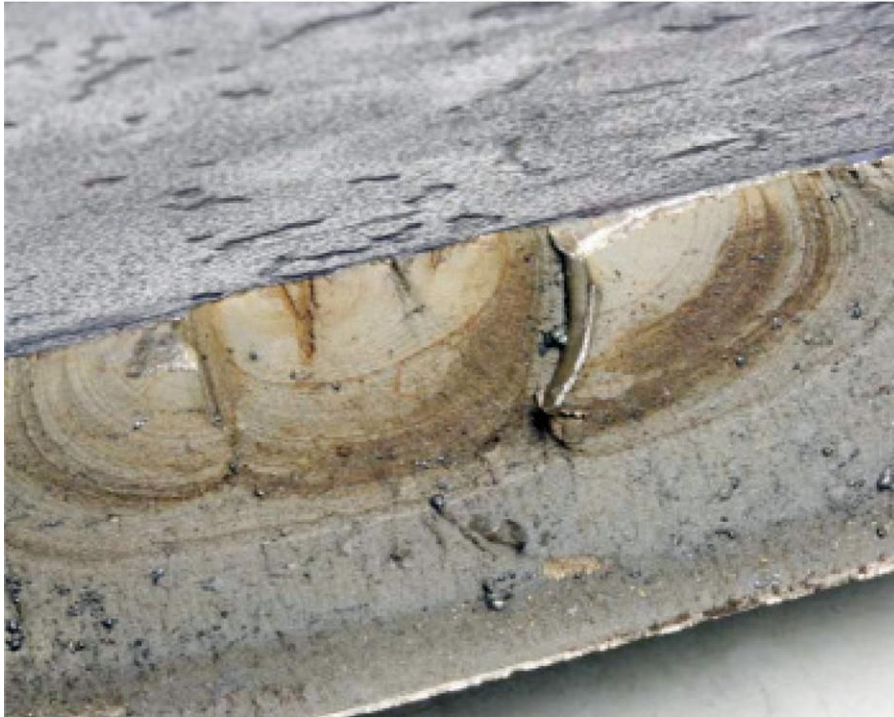
Fig. 3. A crack surface illustrating multiple initiations (origins), each with their own fatigue propagation (Courtesy of Aliya Analytical, Inc.)
