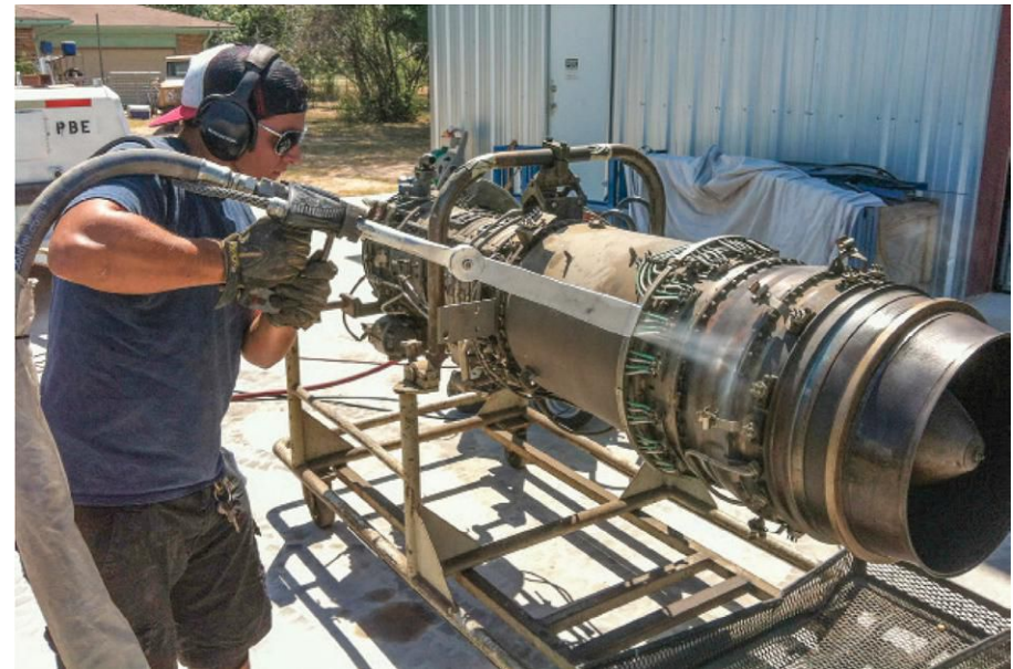
Fig. 2. Portable ice-blasting machine
