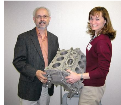
Fig. 2. All-magnesium, six-cylinder engine block developed by the DOE with GM's R&D team
