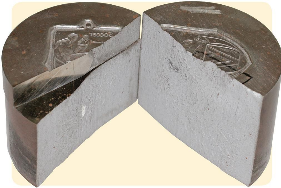
Fig. 1. In-service D2 tool-steel component failure due to quench cracking (Photograph courtesy of Aston Metallurgical Services Co., Inc.)
