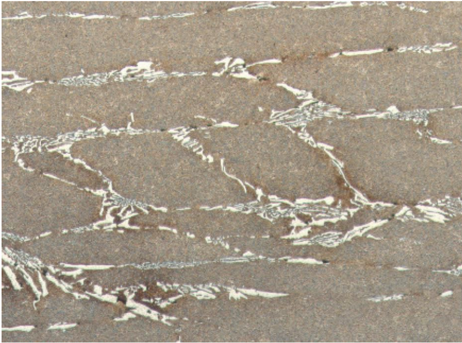
Fig. 3. Hot-working problems on a D2 roll (Photograph courtesy of Aston Metallurgical Services Co., Inc.)
