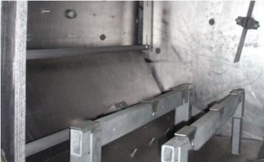
Fig. 5. Typical vacuum-furnace hot zone (Photograph courtesy of ALD-Holcroft)
