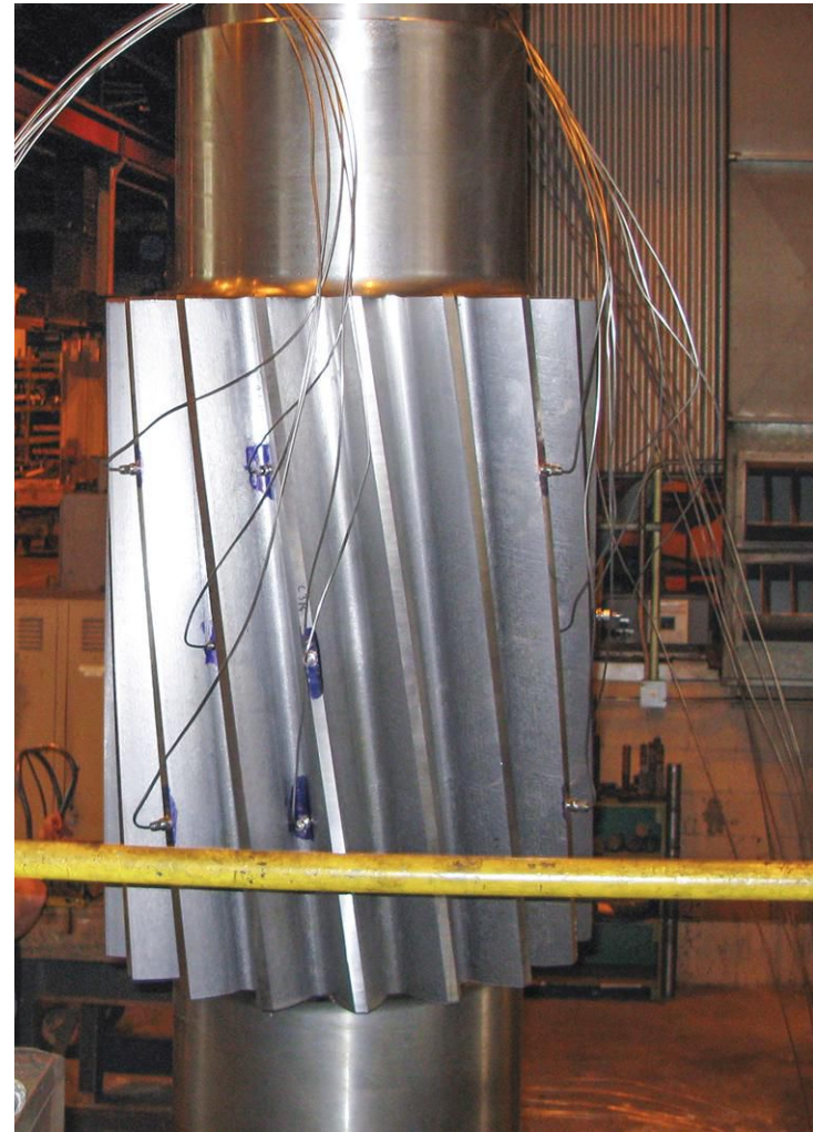
Fig. 1. Test pinion with thermocouples in place
