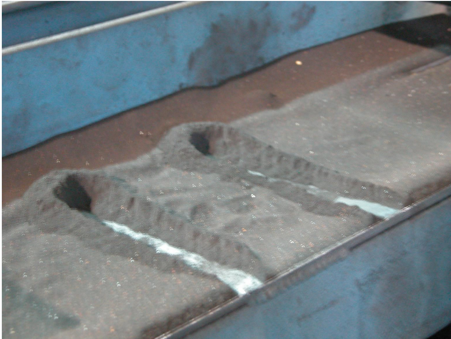
Fig. 1. Soot formation on the front load table of a mesh-belt furnace after one hour with an out-of-control furnace atmosphere
