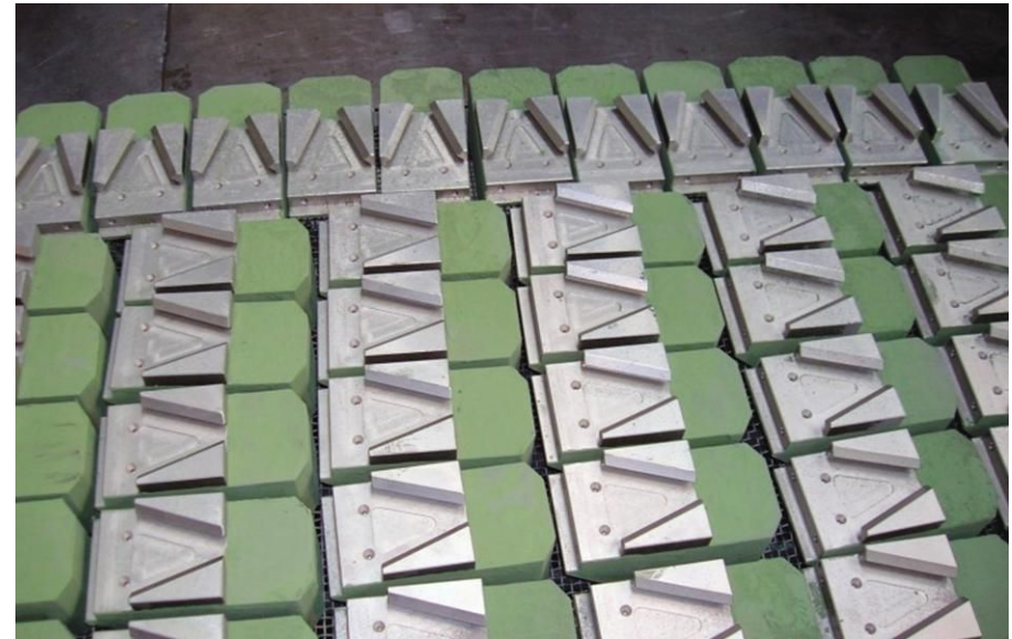
Fig. 2. Tool-steel parts ready for gas nitriding (Photograph courtesy of The Duffy Company and Nüssle GmbH & Co. KG.)
