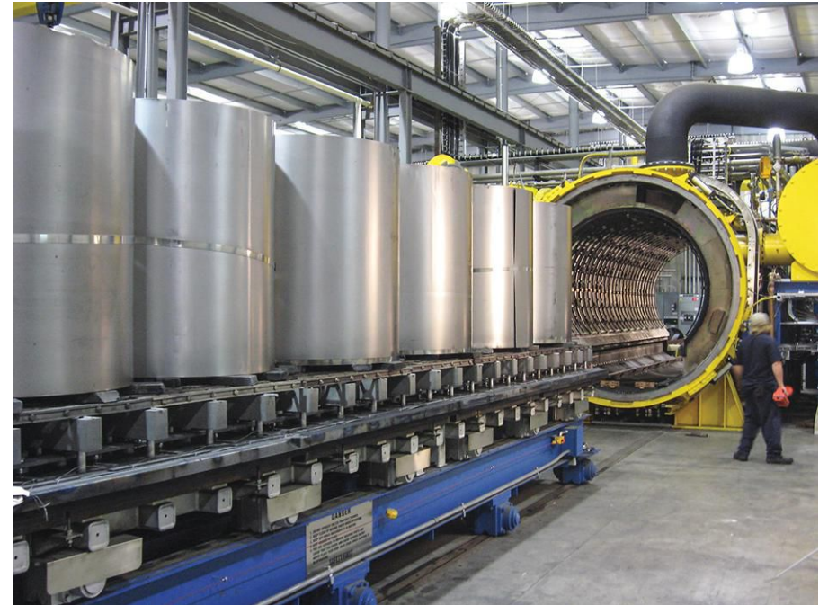
Fig. 1. Load of titanium for vacuum annealing (courtesy of Solar Atmospheres, Inc.)
