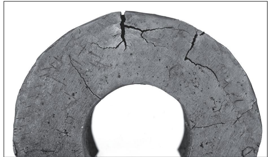
Fig. 1. Section of a cast HH (25% Cr, 12% Ni) stainless steel furnace load-lifting hook that failed due to sigma-phase embrittlement. (Photograph courtesy of George F. Vander Voort, Vander Voort Consulting LLC)
