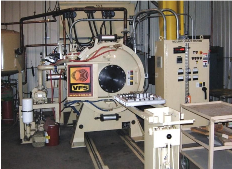
Fig. 1. Typical tool-steel hardening-furnace installation
