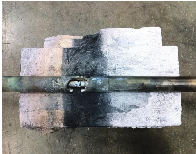
Fig. 2. Oxygen probe and its alloy protection tube destroyed by melting at the exact location of the carbon-rich subsurface layer
