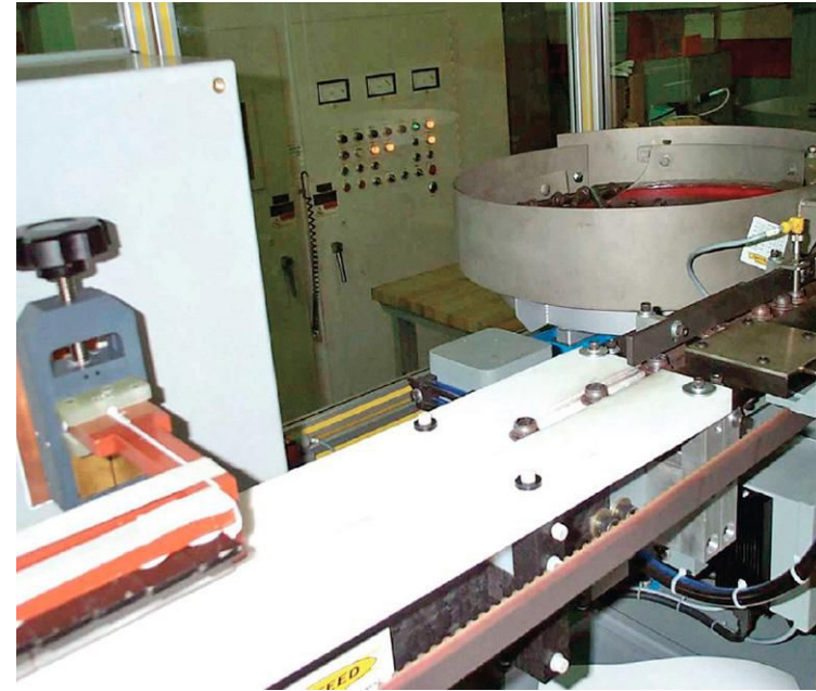
Fig. 4. Induction bolt-head draw system
