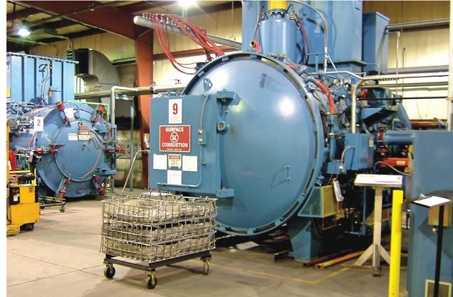
Fig. 7. Typical vacuum-furnace application (Photograph courtesy of Specialty Heat Treating, Inc.)
