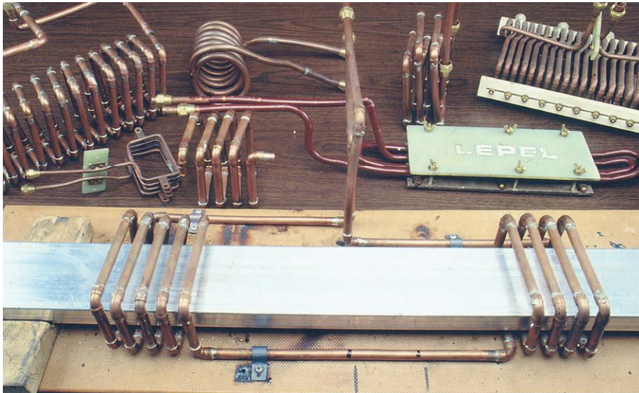
Fig. 3. Typical induction coils used in the RHT process
