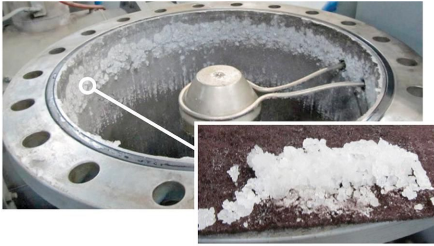
Fig. 1. Contaminated diffusion pump
