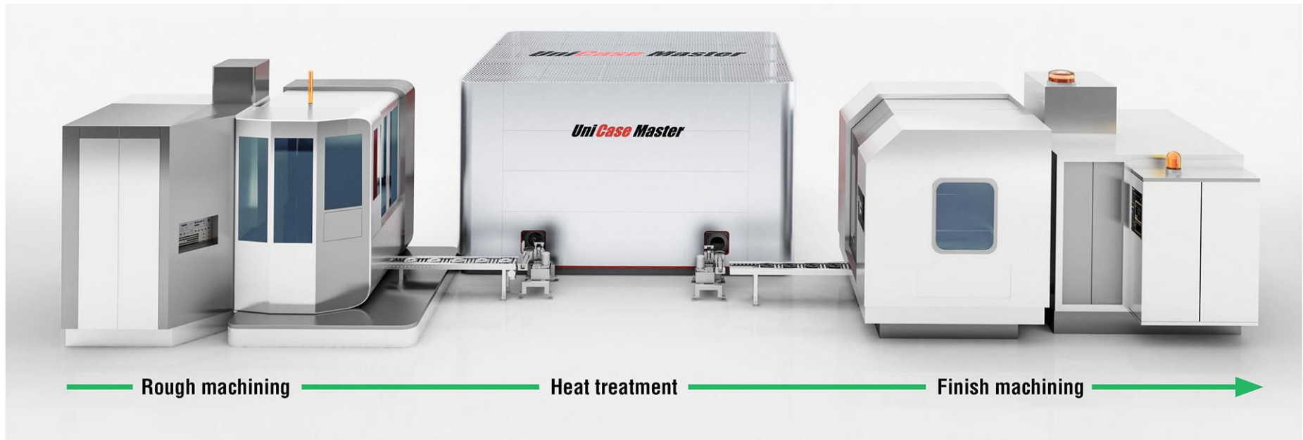
Fig. 2. Integration of heat treating into true single-piece-flow manufacturing (courtesy of SECO/Vacuum Technologies, LLC)
