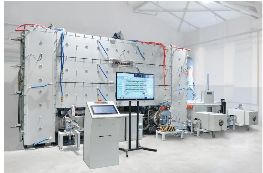
Fig. 2. UniCase Master® in operation months carburizing gears.
