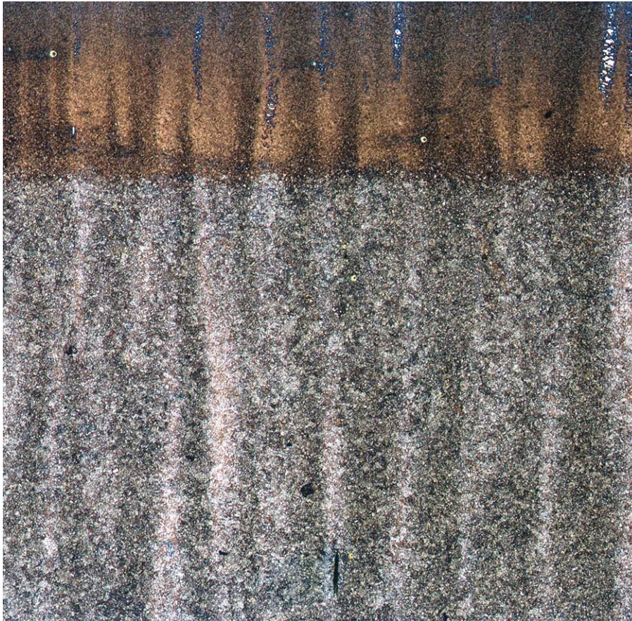
Fig. 2. Banded 4340 microstructure (50x, Vilella's Reagent)
