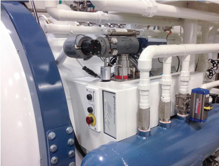
Fig. 2. In-situ mounting of an RGA unit (courtesy of Vac Aero International)
