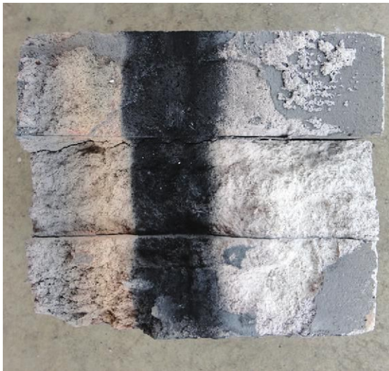
Fig. 1. Carbon-rich subsurface layer inside a refractory wall
