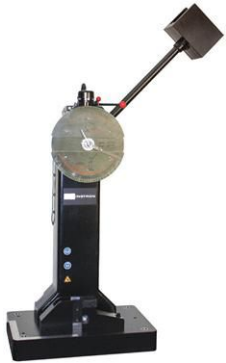
Fig. 3. Instrumented impact pendulum system for Charpy testing (courtesy of Instron)
