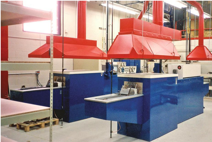
Fig. 6. Typical mesh-belt brazing furnaces (Photograph courtesy of C.I.Hayes)
