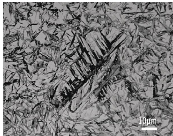
Fig. 4. Plate martensite example (carburized 8620) [4]
