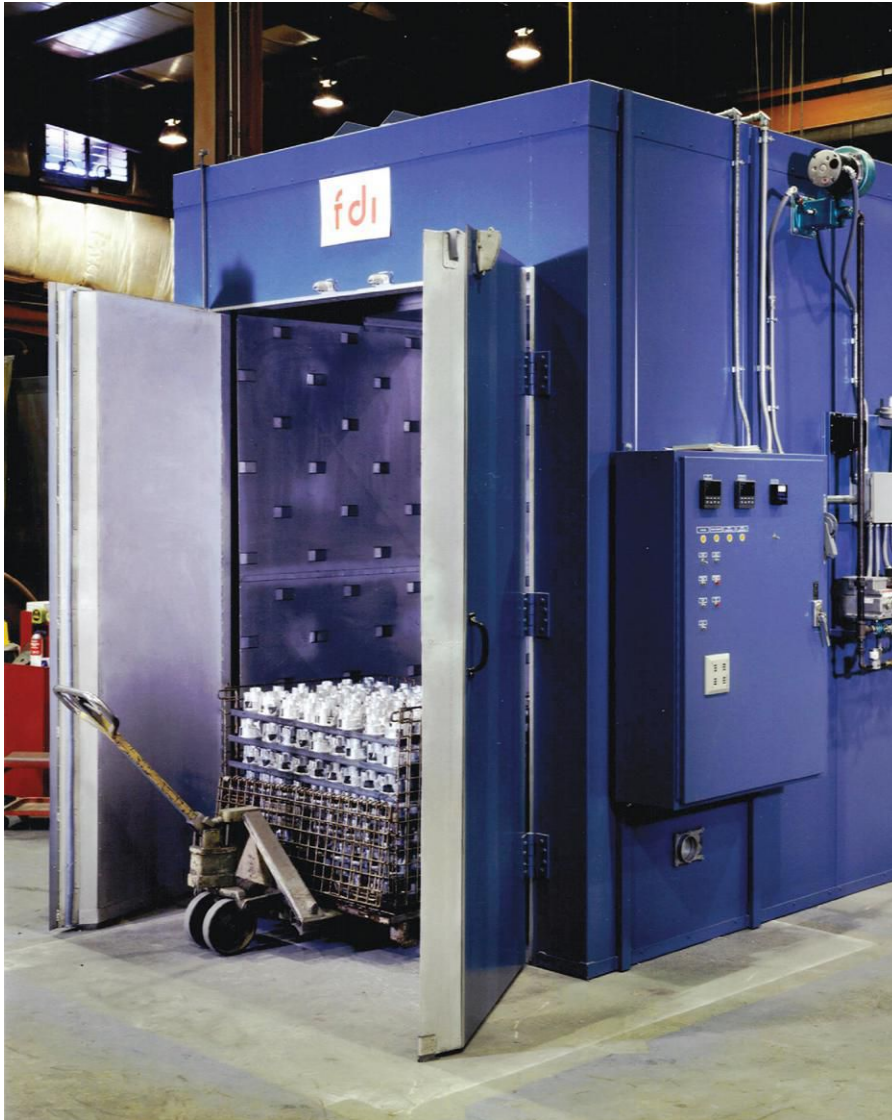
Loading aluminum castings into aging oven. (Courtesy of Wisconsin Oven Corp., East Troy, Wis.)
