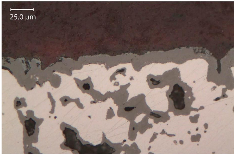
Fig. 1. 4200 steel (0.60%Mo, 0.45%Ni, 0.28%Mn) with 2% Cu and 1% graphite admixed; steam treated for one hour at 575°C (1067°F)
