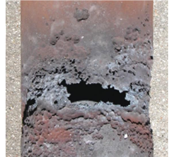
Fig. 3. Alloy radiant tube destroyed by soot accumulation in the insulation
