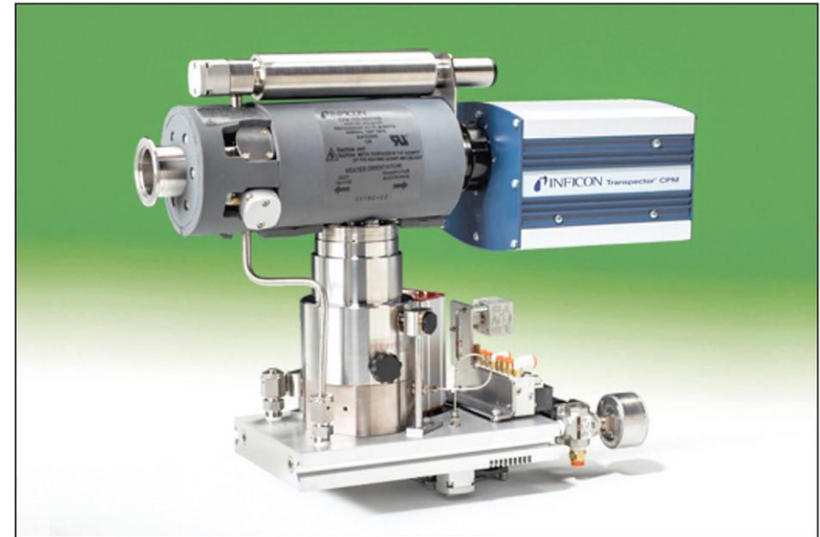
Fig. 1. Residual-gas analyzers (courtesy of Inficon)
