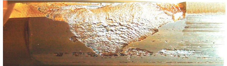
Fig. 3. (above) Gear tooth failure due to spalling (macropitting)
