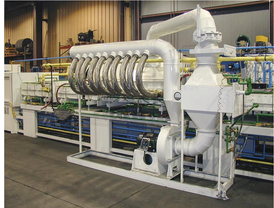
Fig. 1. Cooling-chamber detail on a sinter-hardening furnace (courtesy of Abbott Furnace Company)
