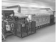
Rotary retort furnace – the 2018 atmosphere heat treatment star
