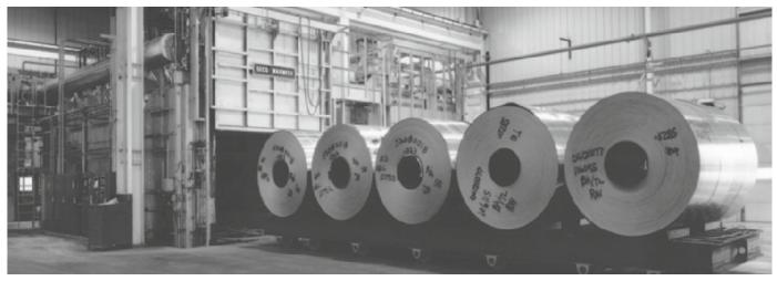
SECO/WARWICK ThermAL's coil annealing multi zone furnaces
