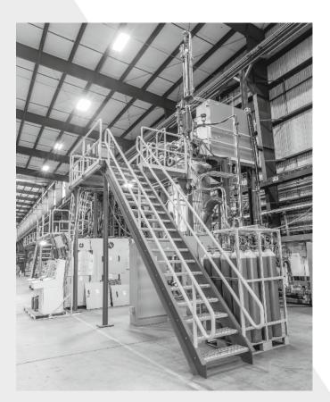
Retech Powder Systems combine induction melting technology and inert gas atomization to allow for a broad range of potential powder sizes of oxygen sensitive metals & alloys. Designed in a range of capacities ranging from laboratory, pilot and production scale, Retech systems are tailored to meet the needs of our customers.
