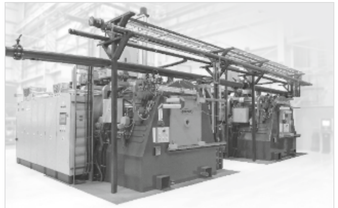
Case hardening by LPC and oil quenching Capacity: 1500 kg, 900x900x1200 mm (WHL) Throughput: 500 kg/h
