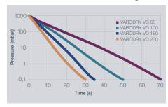
$^*\hbox{+/-}10\%$  tolerance; measurements at operation temperature for a 100l chamber with DN40 pipe and angle valve.
