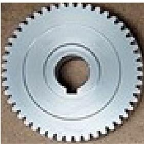
Fig. 4. Gearwheel used in the case hardening process.
