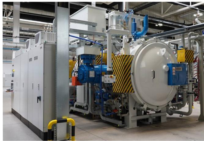
Fig.1. Furnace CMe-T6810-25. On the right – view from the loading side (pre-heating chamber), on the left – view from the unloading side (quenching chamber).
