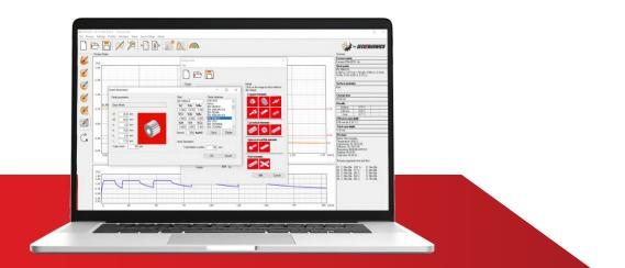
**SimVAC** optimizes the consumption of process gases by adjusting their amount to actual needs. Reducing gas losses and precise carburizing control reduces costs and increases energy efficiency.
