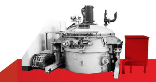
**Pit-LPC** shortens the carburizing process (2-3 times) by eliminating the need to prepare the process atmosphere. This significantly reduces energy and process gas costs. Additionally, the ability to replace up to three atmospheric furnaces with one vacuum solution reduces both investment and operating expenses.
