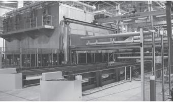
loads are being homogenized. The baffles are adjustable according to the height of the load to effectively limit or block the open space that exists above the load.
