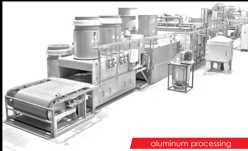
aluminum brazing technology in a protective atmosphere (EV/CAB)
