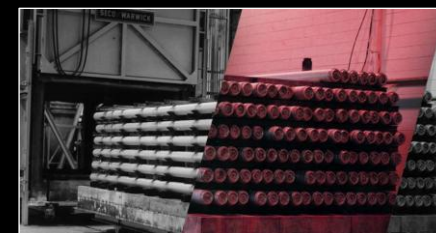
universal chamber furnace for steel hardening and carburizing – Super IQ
