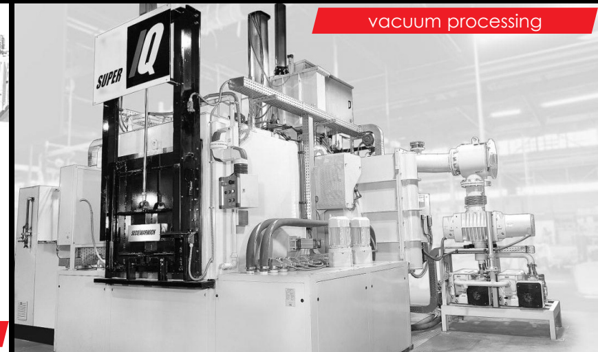
universal chamber furnace for steel hardening and carburizing – Super IQ
