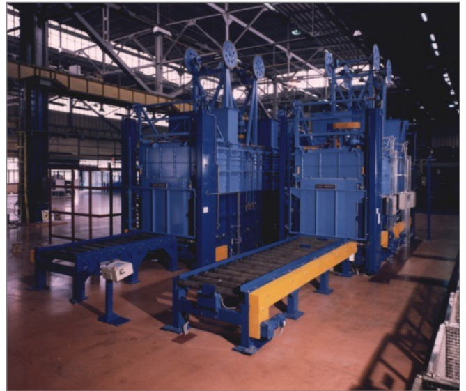
Solution heat treat furnace, front view
