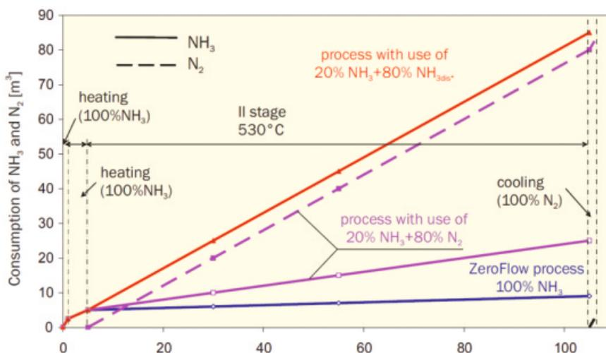
Consumption of  $\text{NH}_3$  and  $\text{N}_2$  in processes with use of double-component atmospheres ( $\text{NH}_3 + \text{NH}_3$  diss. and  $\text{NH}_3 + \text{N}_2$ ) and ZeroFlow®
