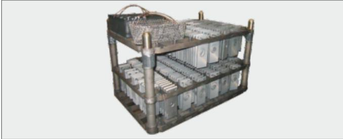
Nitriding of inlet sleeves with the pushing piston, used in molds for aluminium pressure die casting
