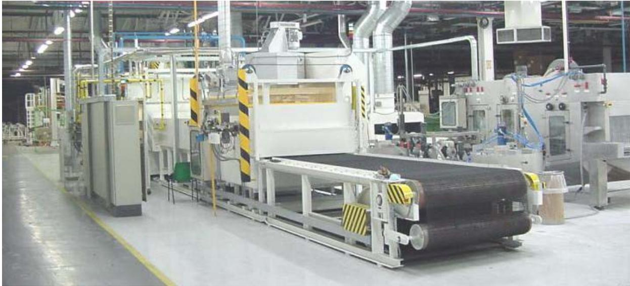
Figure 3 Mesh belt brazing system
