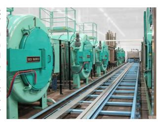
Fig. 1 Picture of the nitrocarburizing system at work
