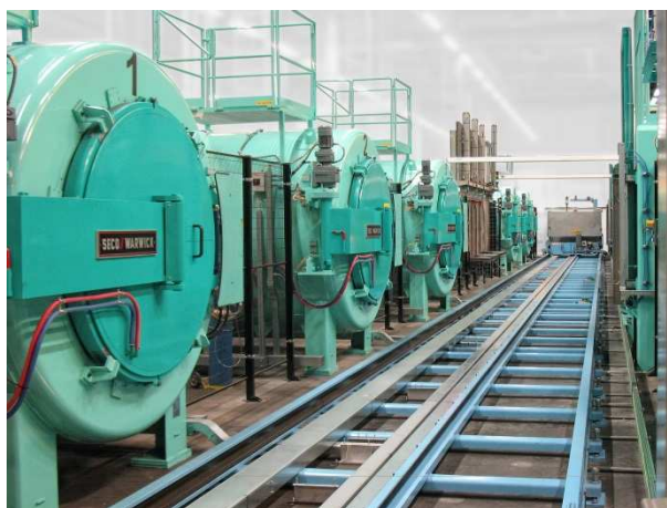
Fig. 1 Picture of the nitrocarburizing system at work
