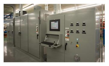
annealing cycle and detect problems the moment they occur. This information and control system provides ABB the ability to produce a stable anneal which is critical to the electrical performance of our products. The new furnace has more than doubled our annealing capacity.
