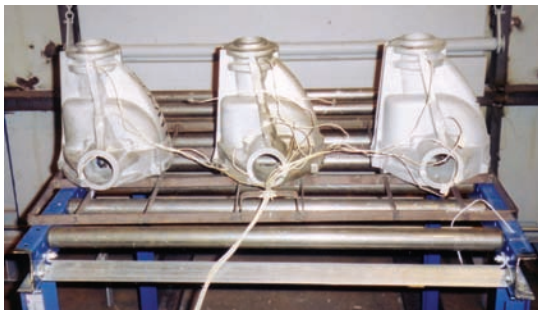
Fig. 5 Test load of Castings
